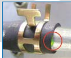
Ultraviolet fluorescent dye highlights the exact location of a leak
